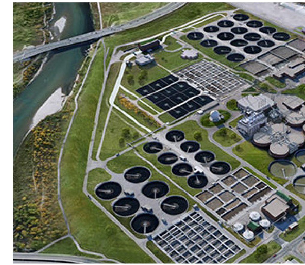
Image: Bonnybrook Wastewater Treatment Plant Bonnybrook converts biosolids from the wastewater into biogas for energy and heat on site.
